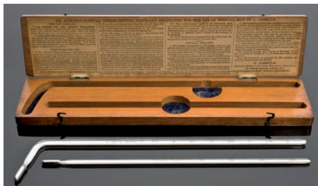
The straight thermometer was 25.4 cm long. The curved thermometer was the shape of a hockey stick measuring 30.5 cm. Both thermometers had a Fahrenheit scale and were carried two in a wooden case under the arm. About five minutes were required for optimal temperature to be reached (Blumenthal).
